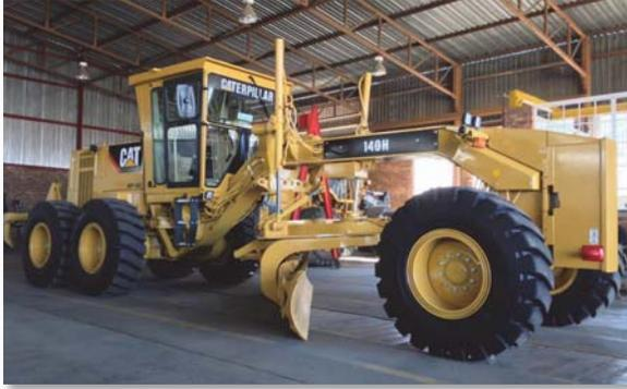
**Grading:** The act of manipulating and leveling the ground surface.
